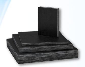
Fabreeka pad is the original "fabric reinforced" bearing pad, used in shock and vibration systems since 1918. The multiple laminations of rubber and fabric allow for large loading with minimal creep and virtually no shape factor associated with unreinforced bearing pad materials.
